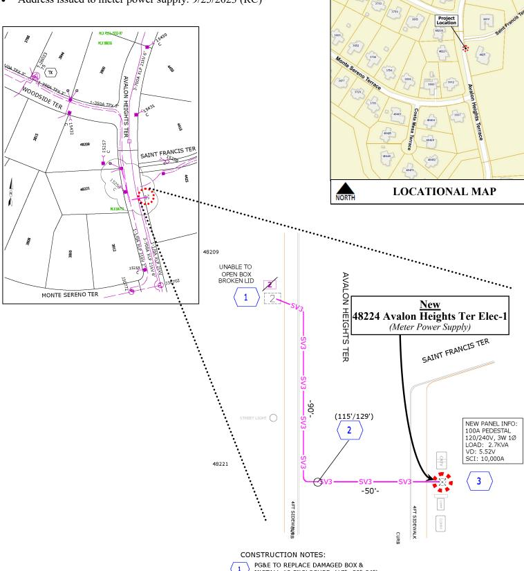
1 PG&E TO REPLACE DAMAGED BOX & INSTALL #2 ENCLOSURE. (17"x 30"x26") INSTALL 6-WAY MULTI-TAPS PG&E CONNECT 1/0A TPX SERVICE CABLE.
